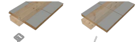
SC-System with screw clip on wooden batten or metal substructure
